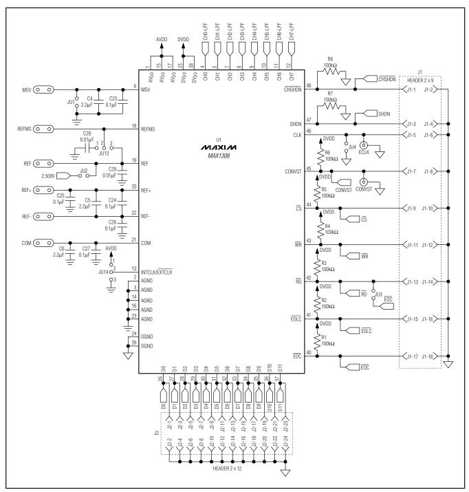
Figure 6. MAX1308 EV Kit Schematic (Sheet 1 of 3)
