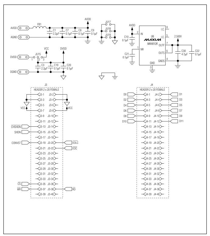
Figure 6. MAX1308 EV Kit Schematic (Sheet 3 of 3)
